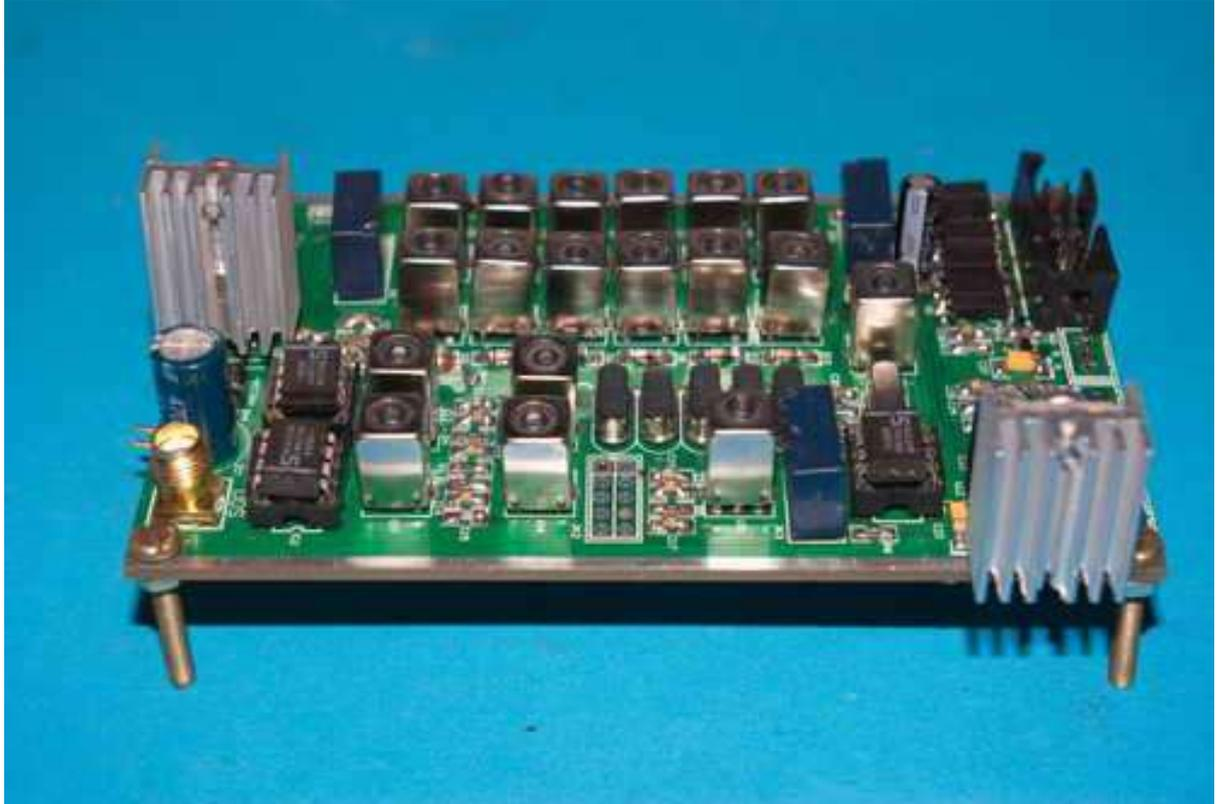
This is an idea to make your boards easier to handle when soldering use nuts and bolts to make temp legs to keep the board level and stable when soldering. This was my first “practice board” I still have to fault find and get this one working. It was also my first attempt at SMT!
